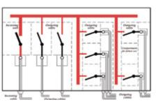
enclosed in their own compartment by means of rigid barriers or partitions. Cable may be glanded elsewhere, e.g. in a common cabling chamber.
