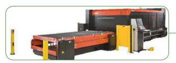
Laser Cutting Capacity: 3050 x 1550 x 200 mm, thickness up to 25 mm (mild steel)
